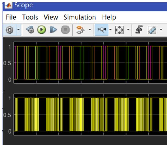
Fig. 5. Coding subsystem and PCM codes
