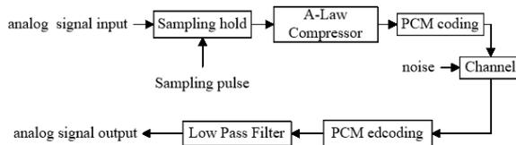
Fig. 1. PCM principle diagram
